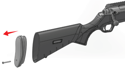
Picture 28: Butt plate is removed from the stock.
